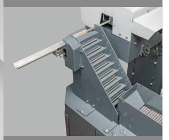
Integrated-type short material feeding mechanism
