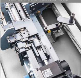
Handwheel Rotation TypeFor bar diameter adjustment.
